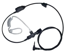
EAS07 Transparent Tube Earpiece with Push-to-Talk Mic
