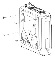
3. Install the repeater on the wall.
